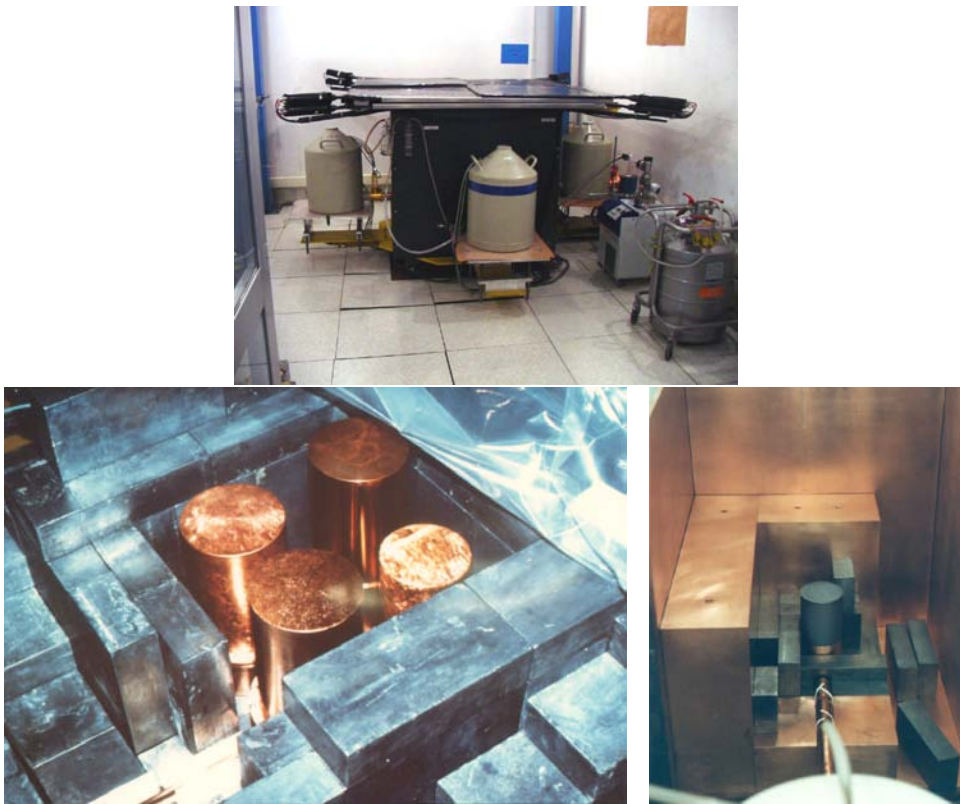
Fig. 1. The HEIDELBERG-MOSCOW \beta\beta -experiment in the Gran Sasso (top), and four of the enriched detectors during installation (bottom left). The fifth detector is installed in an extra shielding using electrolytic copper as inner shield (bottom right).
